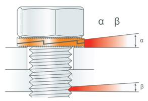
When the bolt and/or nut is tightened the teeth of the NORD-LOCK washers grip and lock the mating surfaces allowing movement only across the cam faces. Any rotation of the bolt/nut is blocked by the wedge effect of the cams. NORD-LOCK safely secures bolted joints exposed to vibration and dynamic loads.
