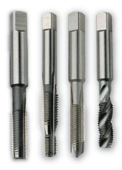
PowerCoil wire thread insert taps are precision manufactured from HSS and are available with Taper, Intermediate and Bottoming leads. Screw Thread Insert (STI) taps have the same pitch but a larger diameter than a standard tap to accommodate the PowerCoil wire thread insert.
