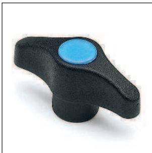
Brass threaded insert. PA: Black reinforced polyamide. Caps on the following colours: grey, orange, black, red, blue, yellow and green, similar to the RAL indicated. (* ) 100u. minimum order quantity.
