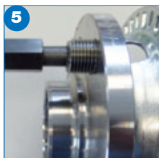
Checking the thread If possible, the ISO thread must be checked for trueness to gauge. The GO thread plug gauge must manually screw in to the complete thread length without application of major force. The No-GO thread plug gauge shall not manually screw into the thread any further than two rotations.
