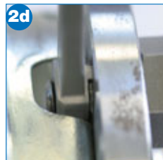
The cheese head screws are tightened with 50 Nm, until the punch lies flat against the thread bush. The thread bush is locked with an open-end wrench, 22 mm. After caulking, the screw joint is loosened and the thread bush screwed out.
