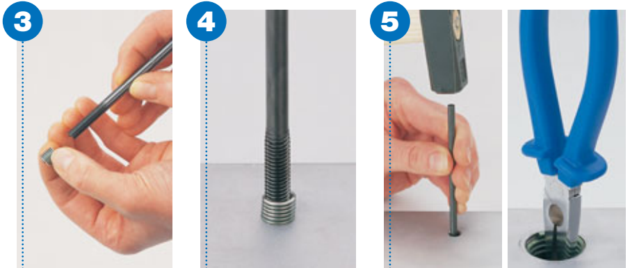
3 Screwing on the HELICOIL® plus
