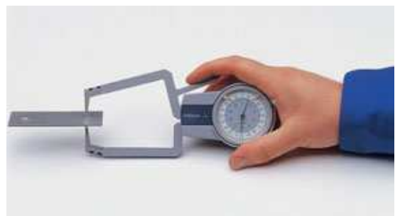
Testing the residual material thickness ST
