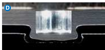
Aluminium 2.45 mm Steel 1.4 mm
